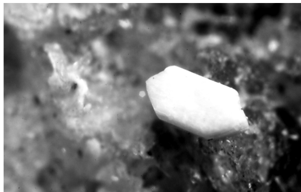
FIGURE 3. Monoclinic dihydrate—Mn(C 2 O 4 )·2H 2 O—pseudomorph after orthorhombic trihydrate Mn(C 2 O 4 )·3H 2 O. Crystal size is about 1 × 0.5 mm and the crystallographic orientation is identical with that in the drawing of Figure 4. Specimen from Falotta, Switzerland.
