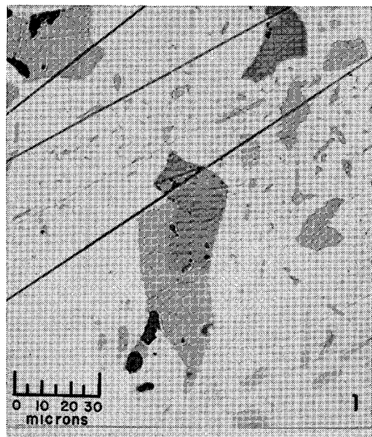
Fig. 1. Photomicrograph of the largest inclusion of ruthenarsenite (light grey) associated with irarsite inclusions (dark grey) in a rutheniridosmine matrix.
