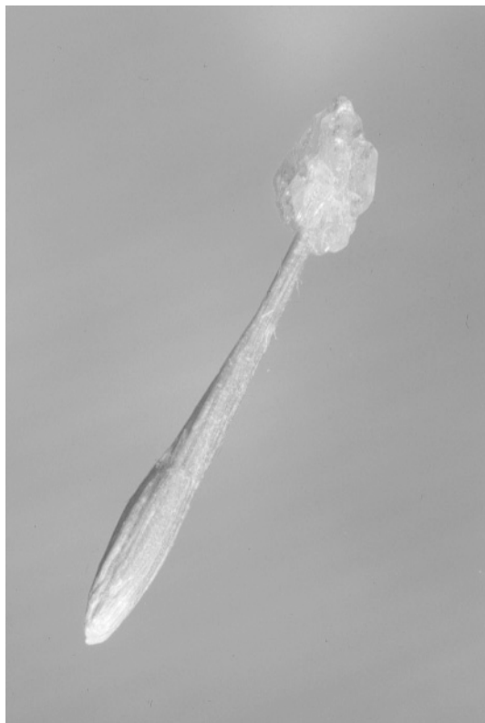
FIG. 3. Photograph of a bundle of walkerite fibers 6 mm in length, capped by hilgardite. Photograph by Q. Wight. Also in color on page 1685.
