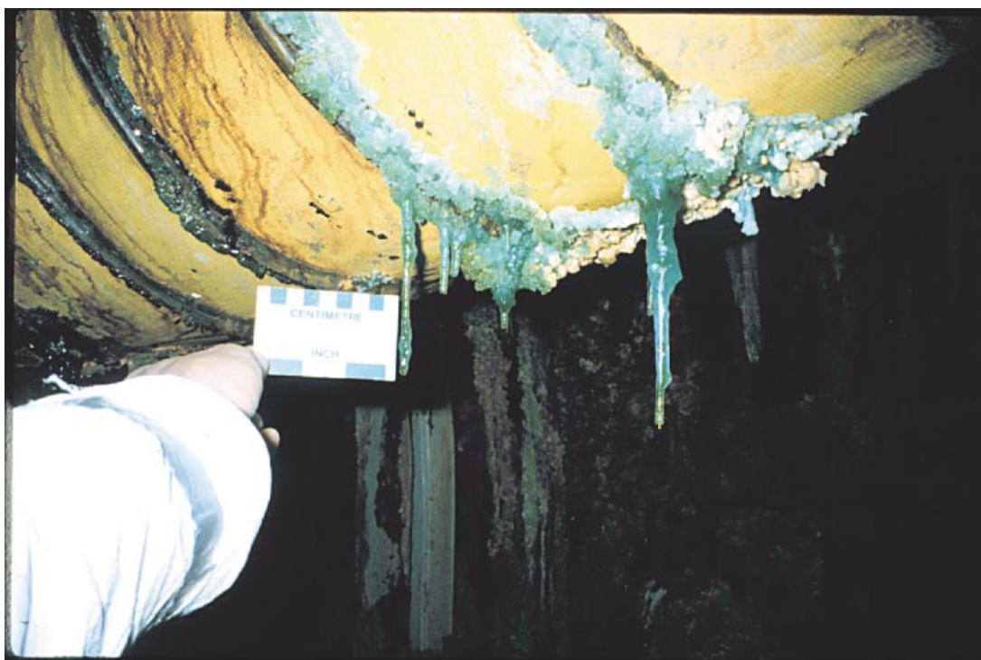
FIG. 3. Smaller stalactites of melanterite forming on a ventilation tube in the same area as those shown in Figure 2. The stalactites are commonly hollow, 3–5 mm in inner diameter, through which fluids pass downward and deposit melanterite at the termination. The stalactite near the scale is an example of such a “drinking straw” morphology.
