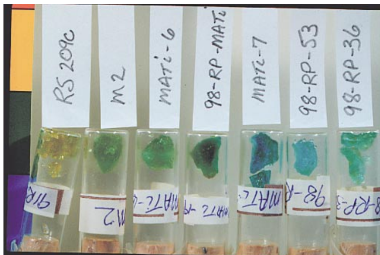
FIG. 5. The variation in color exhibited by melanterite from the Richmond mine. The material shown is the source of crystal fragments used in the X-ray-diffraction experiments. The sample numbers shown are used throughout the paper. The sample vials are 1 cm in diameter.
