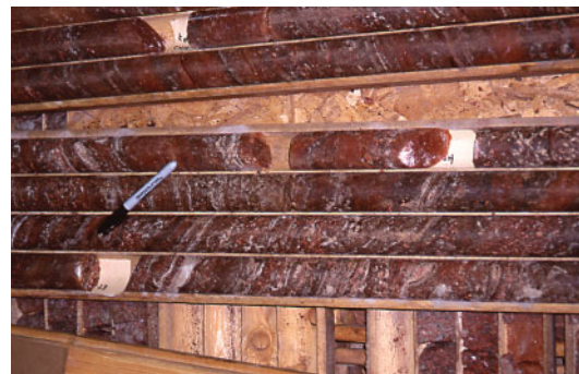
FIG. 3. Photograph of a section of drill core from the Penobsquis deposit. The borate minerals are white spheroids within the orange-colored halite.
