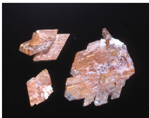
FIG. 15. Photograph of veatchite plates (total width of field of view 12 mm) from the Penobsquis deposit. Photograph by L. Horváth.
