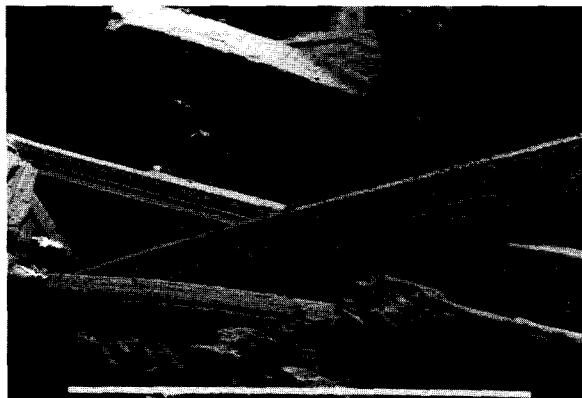
Fig. 1. Acicular scainiite crystals (Scanning electron microscope; scale bar = 1 mm).
