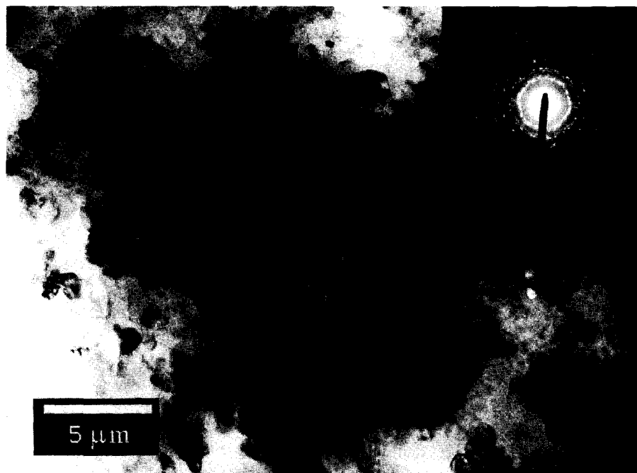
Fig. 1. TEM image showing the typical intergrowth of rodolicoite and grattarolaite; the corresponding electron diffraction pattern is also shown.
