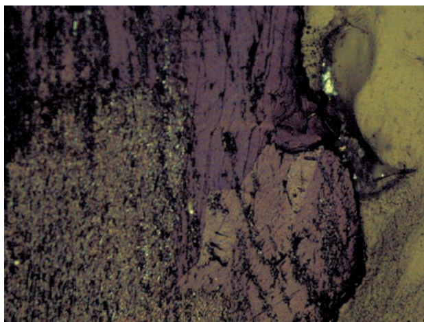
Fig. 231. NM 4807. “Frieseite” crystal parallel with section. Reflected light, crossed polarizers. Magnification 200 \times .
