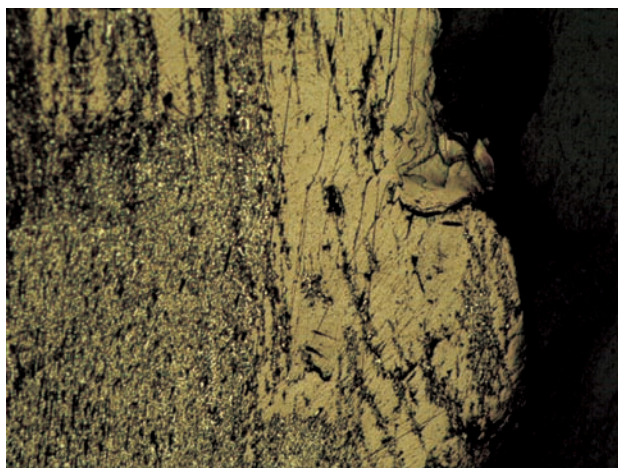
Fig. 230. NM 4807. “Frieseite” crystal parallel with section. Reflected light, single polarizer. Magnification 200 \times .
