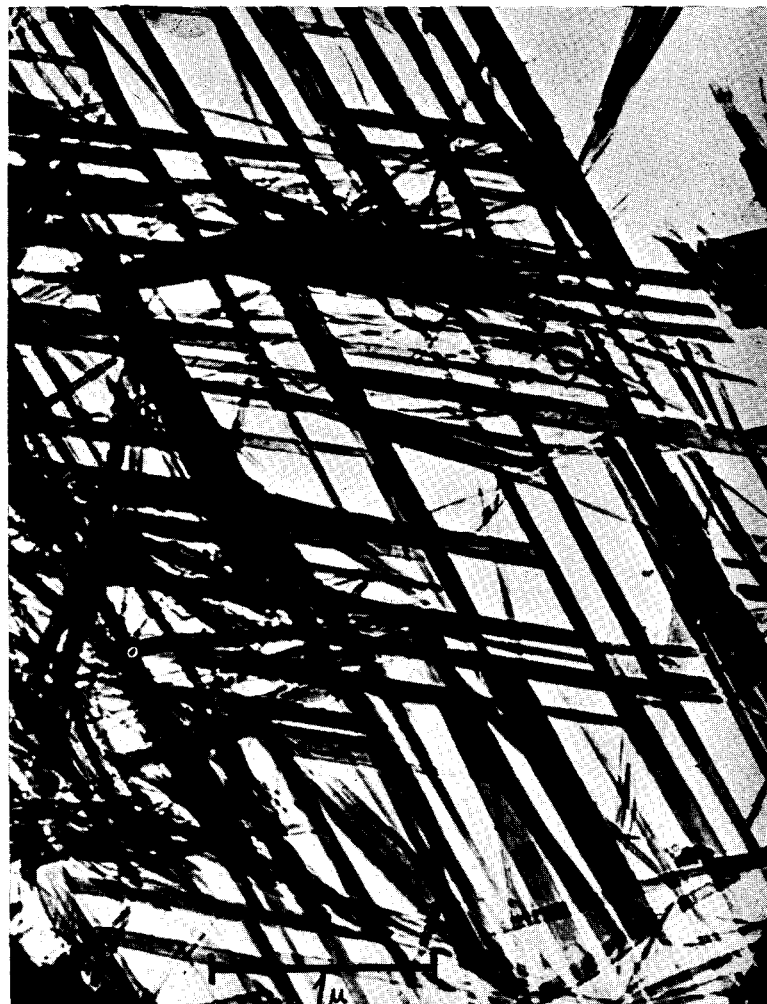
FIG. 2. Electron micrograph of a mat showing two texture axes for the \beta -FeOOH crystals composing it, which had transformed in the solid from \text{FeCl}_2 \cdot 4\text{H}_2\text{O} .
