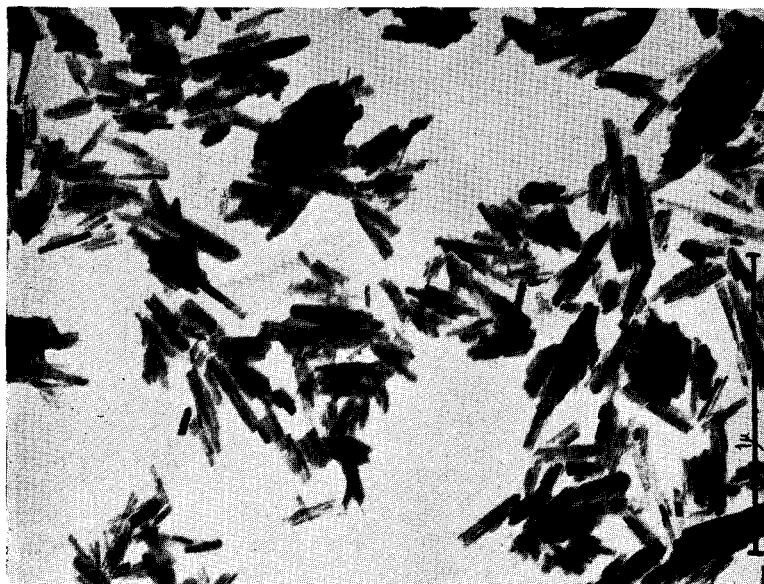
FIG. 1. Electron micrograph of crystals of akaganéite.
