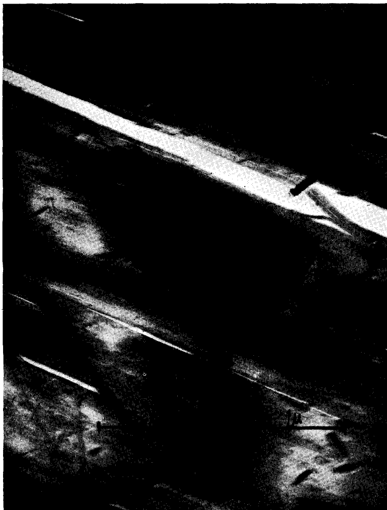
FIG. 3. Electron micrograph of a sheet of \beta -FeOOH fibres produced by a solid transformation from \text{FeCl}_2 \cdot 4\text{H}_2\text{O} .
