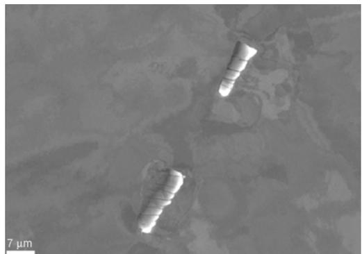
FIG. 4. BSE image (orientation contrast) showing the fragmented platy CrN crystals in deformed kamacite.
