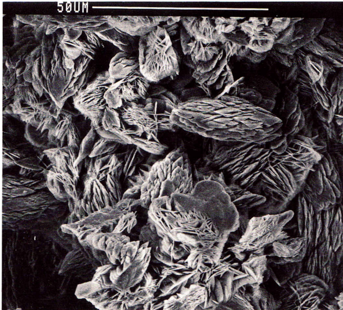
Figure 2. Scanning electron photomicrograph of a vug containing edgarbaileyite crystal aggregates (Socrates mine).
