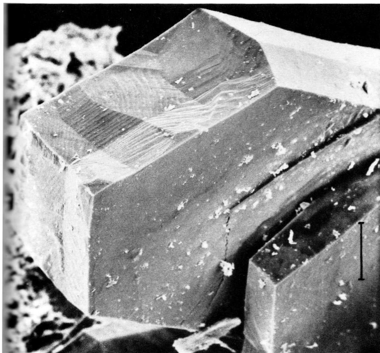
Figure 4. (left) A scanning electron micrograph of a single, large jonesite crystal. Faces other than the \{010\} pinacoid are \{310\} and \{2\bar{1}0\} . X-ray diffraction and goniometric measurements prove that the re-entrant faces are not a result of twinning, but from the rapid growth of the \{010\} faces. Length of the bar is 0.1 mm.
