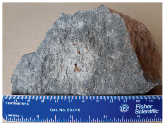
FIG. 4. Hand sample of the grey phonolite with millimeter-sized vesicles containing radial aggregates of windmountainite (reddish-brown, acicular). Note the bleached haloes (white) that surround the vesicles; these extend up to 8 mm from the vesicle margin. The brown area on the right of the sample represents surface weathering.
