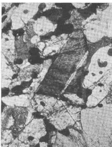
FIG. 8. ( \times 56 .) Composite twin of alleghanyite taken with crossed nicols. The twin-planes are (001) and (305).
