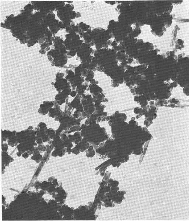
FIG. 14. Electron micrograph of Mn_3O_4 partially oxidized to \gamma -MnOOH (needles). \times 80,000 .
