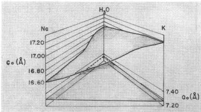
FIG. 3. Plot of the effect of composition on the cell parameters of natural and synthetic jarosites, natrojarosites and hydronium jarosites.
