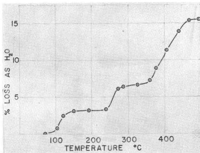
FIG. 1. Weight loss as a function of rising temperature in synthetic jarosite. Each temperature point has been maintained for 24 hours.
