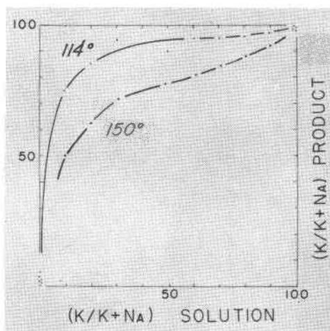
FIG. 4. Relationship of alkali content in starting solution and the resultant jarosite product as a function of temperature. Increasing temperature (and pressure) also reduces the hydronium ion content of the product.
