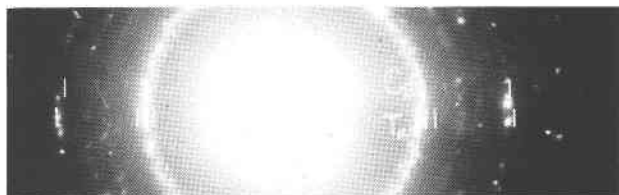
FIG. 8. Diffraction pattern from initially amorphous opal from Andamooka (S1) after being heated to 1200°C for 3 hours. This diffraction pattern comes from an area containing many fragments.
