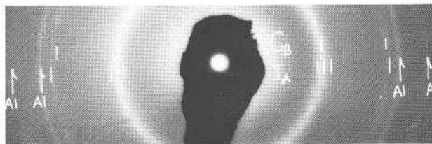
FIG. 4. Diffraction pattern of a sample from Mt. Bougrom, Queensland (V5) together with 111 and 200 rings from aluminium. The most intense lines from cristobalite ( C\beta ) and tridymite ( T\alpha ) are marked.
