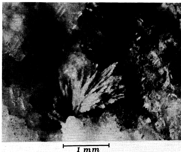
Fig. 1. Tuft in the center of the photograph is composed of platy crystals of jervisite and cascandite.
