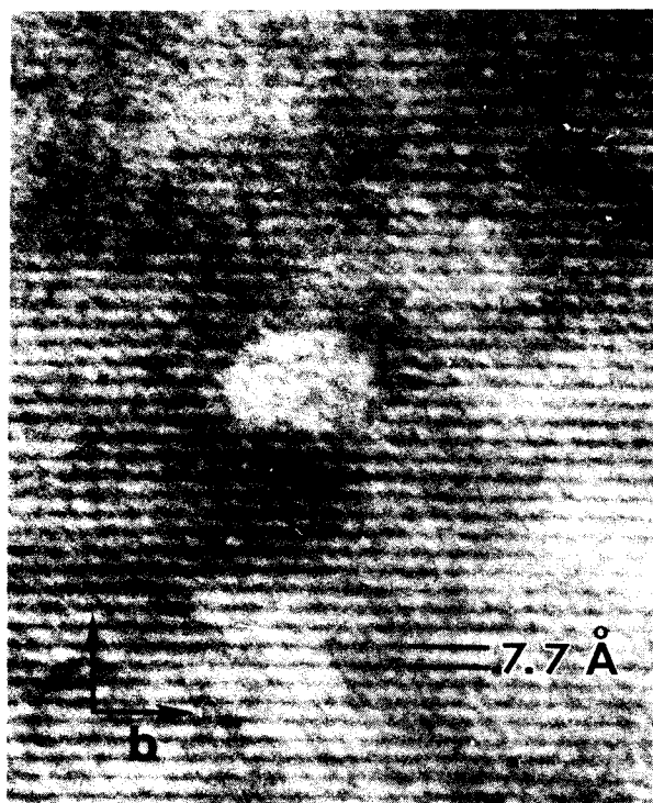
Fig. 4. High-resolution TEM image showing fringes arising from the well-ordered 7.7 Å superstructure in aged K/Na-birn.
