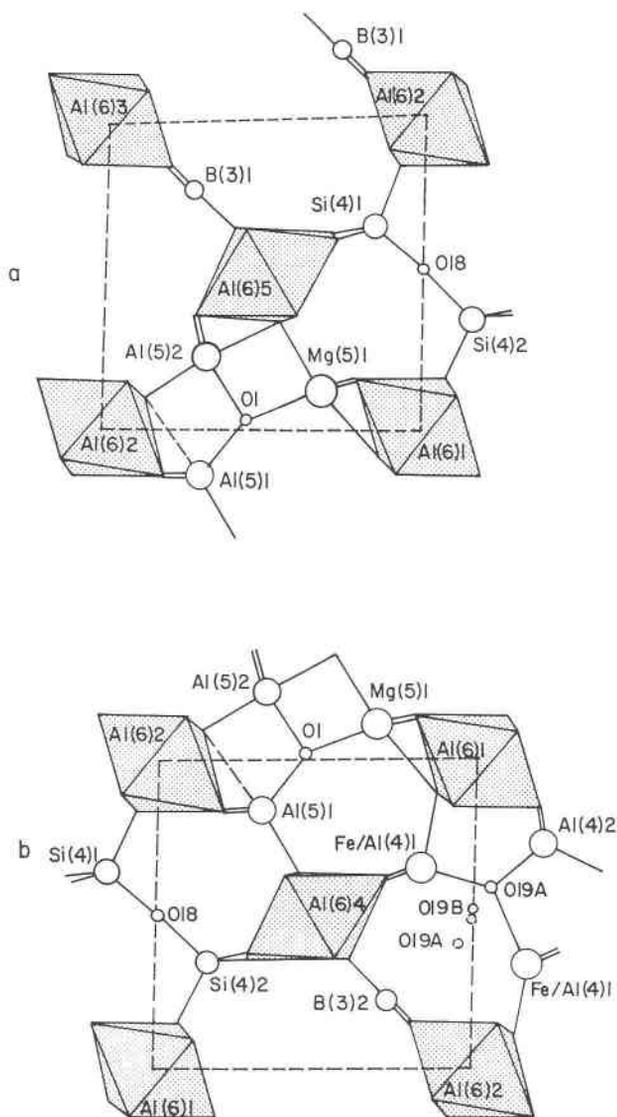
Fig. 3. Two mullite-like constituent slabs of the werdingite unit cell, each bounded by Al octahedra in the corner chains, and containing four of the 16 bridging cation sites. (a)  $\text{Al}_2[\text{MgAlBSi}]\text{O}_6$  slab. (b)  $\text{Al}_2[\text{Al}(\text{Al,Fe})\text{BSi}]\text{O}_{6.5}$  slab. The long fifth bond to Al(5)1 is shown by a dashed line. In the adjacent slab to the right, B in B(3)2 has been replaced by Al in Al(4)2.
