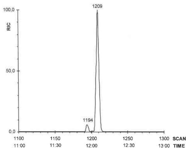
FIGURE 1. Gas chromatogram of original hartite crystals indicating high chemical purity of the material studied. The smaller peak at scan 1194 corresponds to an admixture that is 4.31% of the total weight amount.
