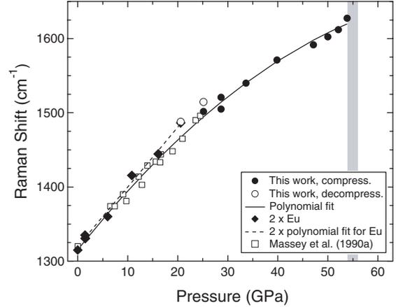
**FIGURE 4.** Pressure induced shift of 1320 cm<sup>-1</sup> mode. Notation is the same as in Figure 3. The solid diamonds and dashed line shows twice the frequency of the  $E_u(\text{LO})$  mode.
