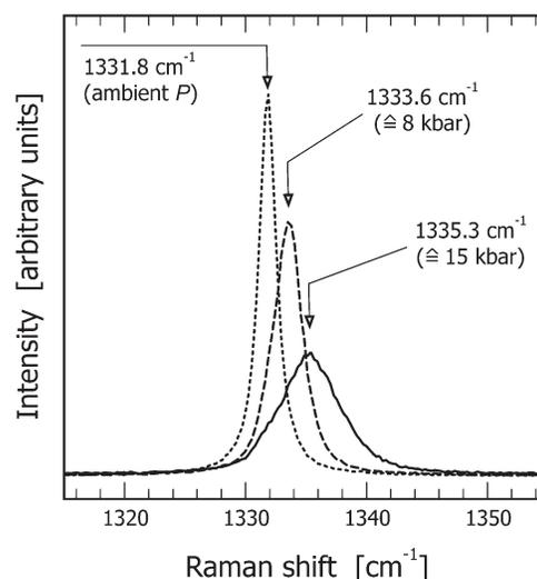
FIGURE 1. Raman spectra of three micro-areas at the surface and inside diamond specimen PAG12. Increased remnant pressure (compressive strain) is indicated by the increased Raman shift of the diamond  $LO=TO$  phonon. Remnant pressures were assigned based on the calibrations of Grimsditch et al. (1978) and Sharma et al. (1985).
