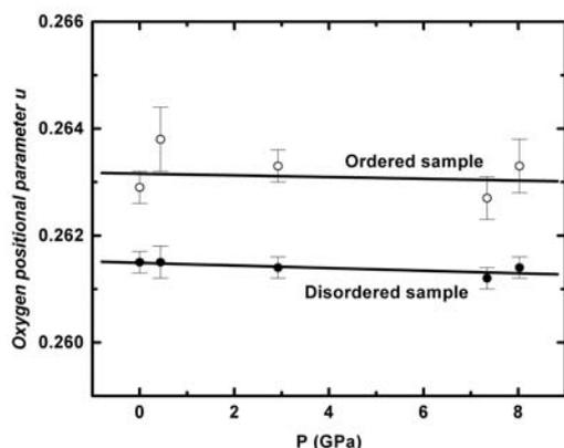
FIGURE 2. The oxygen coordinate  $u$  as a function of pressure for ordered (ord) and disordered (dis) spinels investigated in this study. Symbols as in Figure 1. The solid lines are weighted linear fits through the data resulting in the following equations:  $u_{(\text{ord})} = 0.2634(3) - 0.00004(1) P$  (GPa) and  $u_{(\text{dis})} = 0.2614(1) - 0.00002(1) P$  (GPa).
