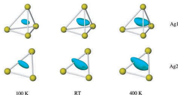
**FIGURE 4.** Non-harmonic probability density isosurfaces of Ag1 and Ag2 for samsonite at 100 K, RT, and 400 K. The size of the S atoms is arbitrary. Level of the 3D maps:  $0.03 \text{ \AA}^{-3}$ .
