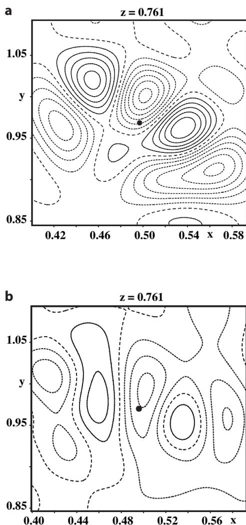
FIGURE 2. Difference Fourier maps for samsonite at RT, centered on Ag2 (label). Contour lines in intervals of  $0.5 e^{-} \times \text{\AA}^{-3}$  for positive values (continuous lines) and negative values (dashed lines). (a) Second-order tensor (classical anisotropic parameters) and (b) third-order atomic displacement tensor for Ag2.
