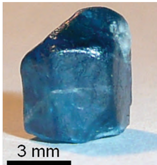
FIGURE 2. The apatite crystal used for the neutron diffraction experiment.
