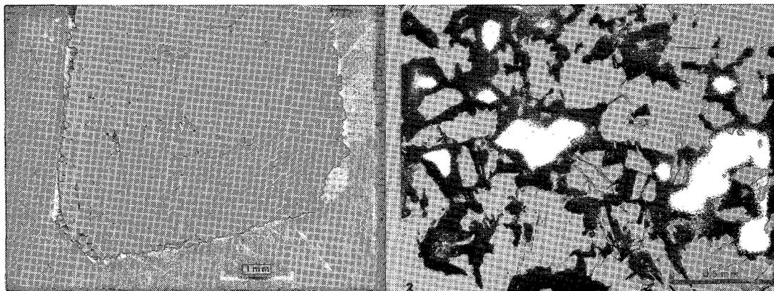
FIG. 1. Polished section of a euhedral bipyramidal crystal of hafnian zircon in epoxy mount, oriented roughly parallel to  $c$  (sample ZH-1). Two stages of alteration, marked by progressively darker color, reveal a growth-zoning pattern by selective attack.
