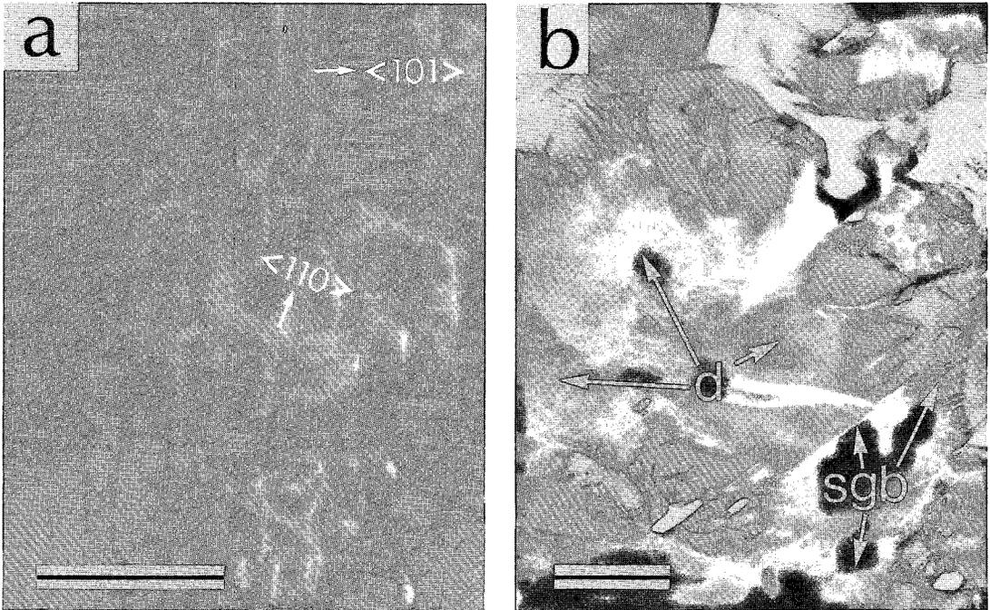
FIG. 6. Defect microstructures. Scale bars: 1  $\mu\text{m}$ . a) Dislocations at twin front imaged near (111) with bowed segments perpendicular to expected slip directions  $\langle 101 \rangle$  and  $\langle 110 \rangle$ . b) Deformation substructure resulting from dislocation walls defining subgrain boundaries (sgb), which in turn contain free dislocations (d). Subgrain boundaries are parallel to traces of (110) and (101).
