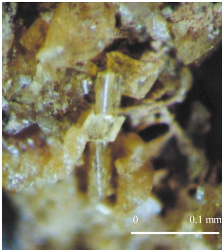
FIG. 2. An aggregate of pale yellow crystals of ushkovite.
