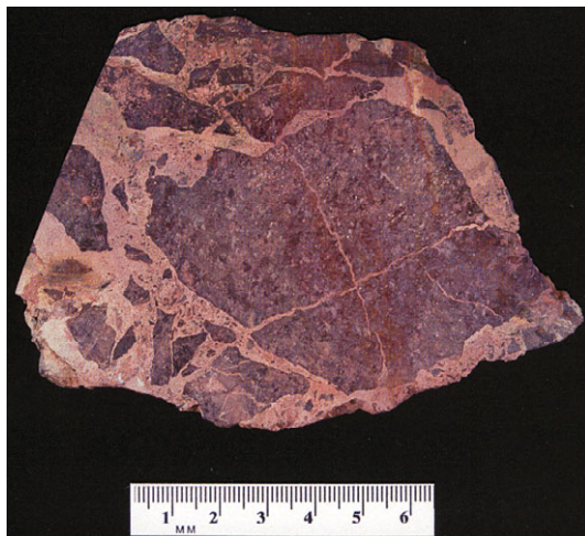
FIG. 2. Altered breccia, sample SL 35. Dravitic tourmaline comprises as much as 20% of the matrix. Marked divisions are centimeters.
