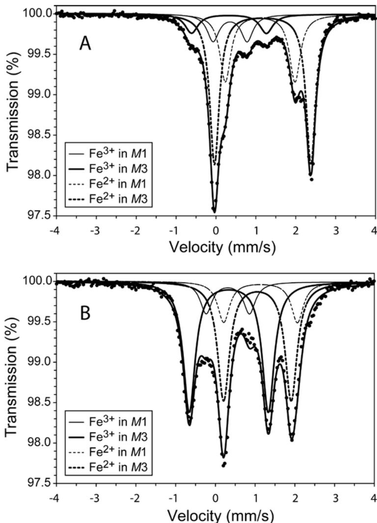
FIG. 18. Fitted Mössbauer spectra for dollaseite-dissakisite. (A) Sample #270427 from Östanmoora. (B) Sample 540027 from Malmkärra.
