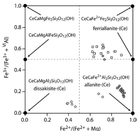
FIG. 19. Compositional diagram for allanite-(Ce) and related minerals from subtype-1 deposits. Filled symbols: Rödbergsgruvan, open symbols: Bastnäs. Analytical results for ferriallanite-(Ce) from Bastnäs, presented in Holtstam *et al.* (2003b), are included.
