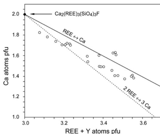
FIG. 9. Compositional diagram showing the variation of Ca versus REE + Y in fluorbritholite.
