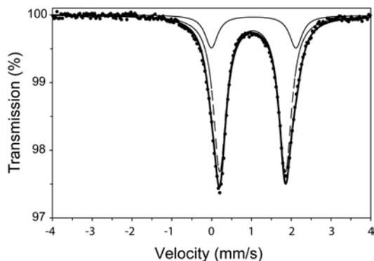
FIG. 15. Fitted Mössbauer spectrum for gadolinite (sample #970319 from Malmkärra).
