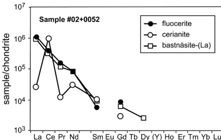
FIG. 3. Chondrite-normalized REE patterns of fluocerite and its alteration products, from the Bastnäs deposit.
