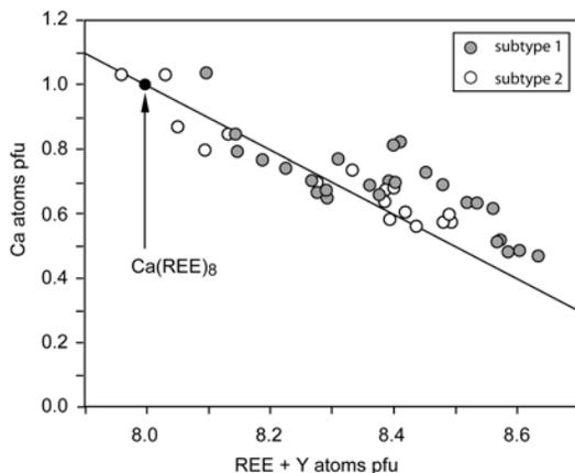
FIG. 6. Compositional diagram showing the variation of Ca versus (REE + Y) in cerite-(Ce). The straight line corresponds to an ideal REE + Y + Ca = 9 *apfu*.
