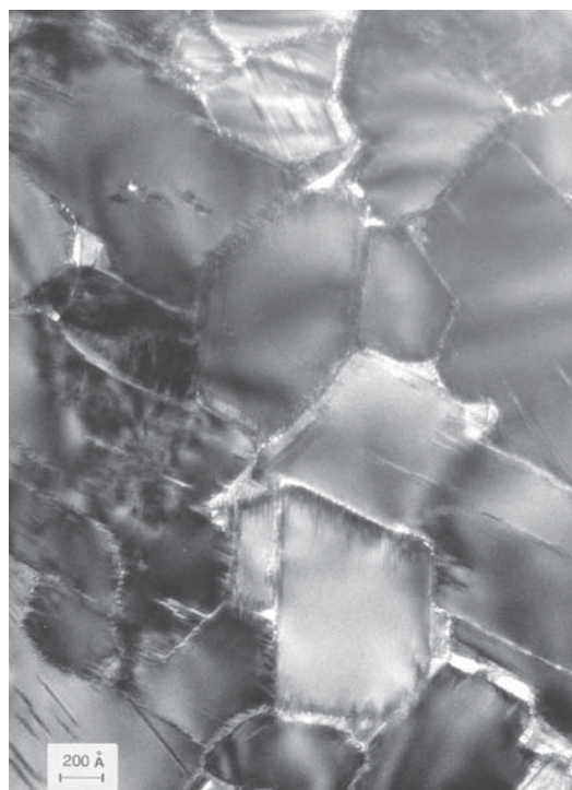
FIG. 2. Medium-resolution TEM image of carlosturanite fibers in sample 128, as seen along the fiber axis, i.e. , the [010] direction.
