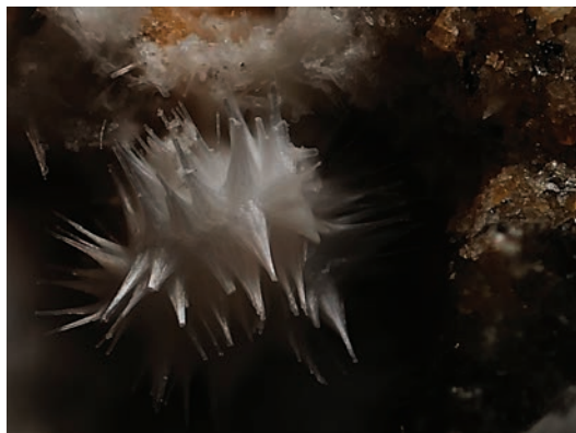
FIG. 1. Aggregates of acicular crystals of kottenheimite (white), with earlier melilite crystals, on cuspidine. Field of view: 1.2 mm.
