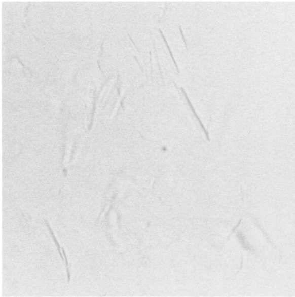
FIGURE 1. Talc flakes in 1.584 refractive index liquid. Note that there are particles in this field that have aspect ratios greater than 3:1. Width of view 0.13 mm.
