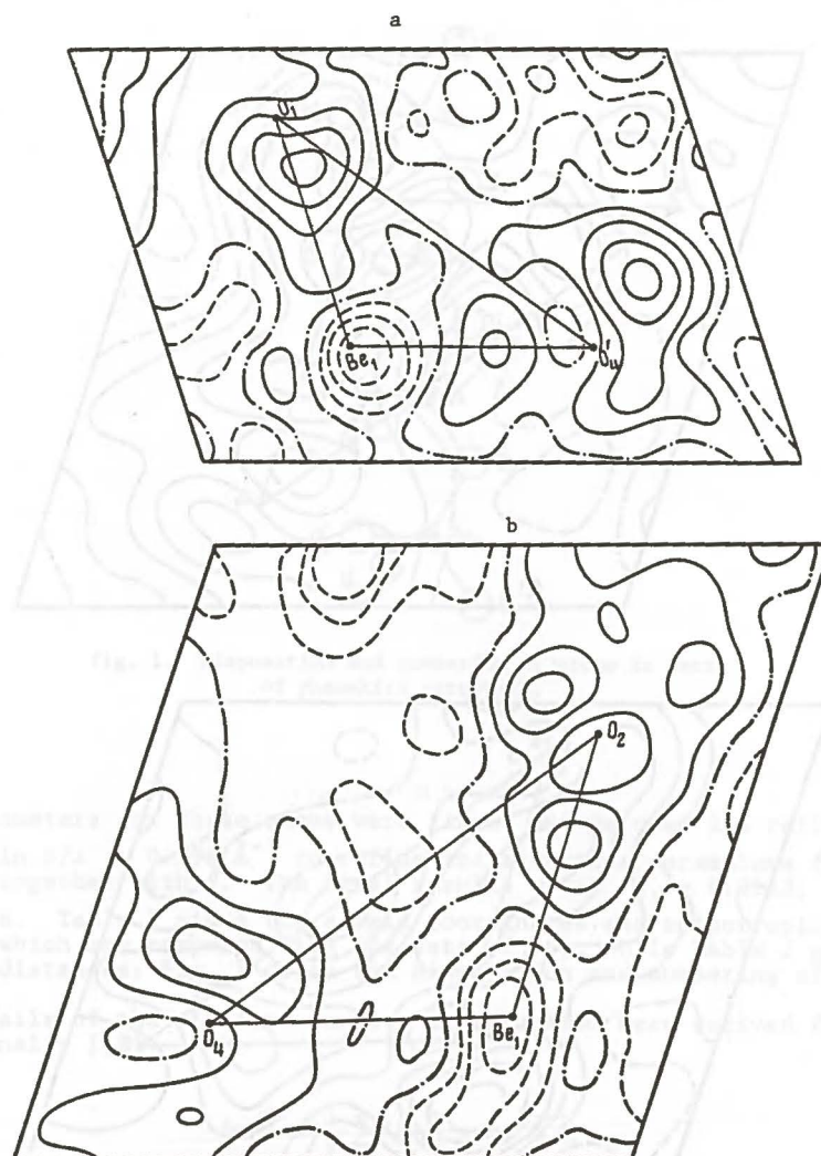
Fig. 3. 2D-DEDD maps of planes of the Be 1 tetrahedron containing O 1 -Be 1 -O 4 (a) and O 2 -Be 1 -O 4 (b). Intervals between lines: a) 0.09 e·Å -3 ; b) 0.08 e·Å -3 .
