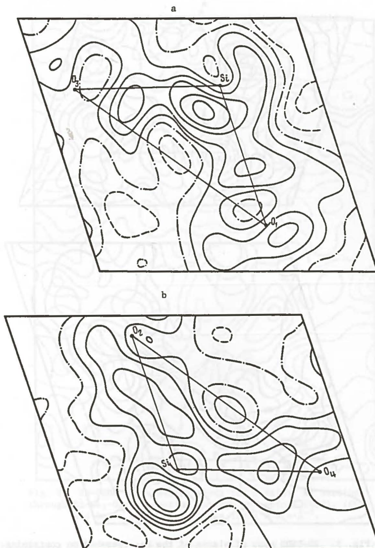
Fig. 2. 2D-DEDD maps of planes of the Si tetrahedron containing O_1 -Si- O_3 (a) and O_2 -Si- O_4 (b). The solid lines here and subsequently join points having excess deformation electron density, while the dashed lines join ones with deficient density, and the dot-dash lines are those of zero density. Intervals between lines 0.1 \text{ e} \cdot \text{\AA}^{-3} .
