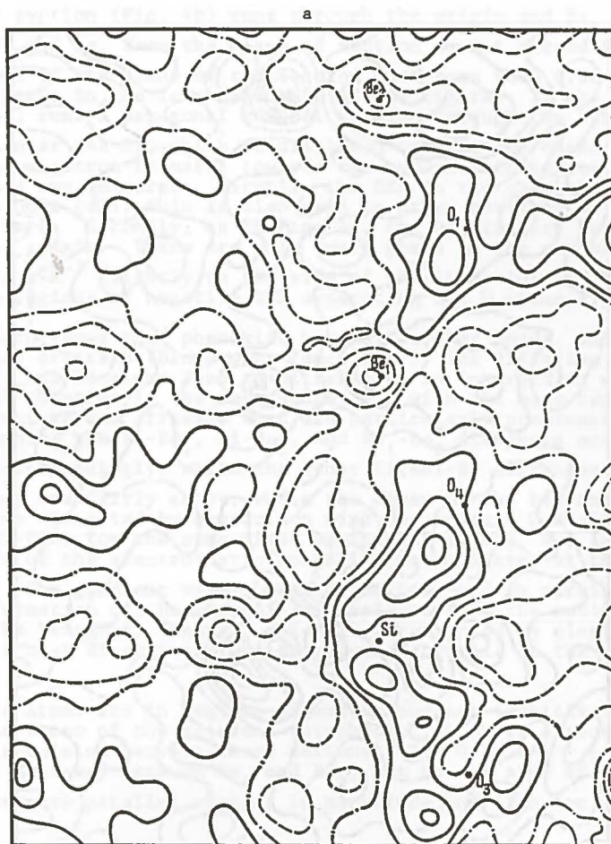
Fig. 4. 2D-DEDD maps passing along the c axis: a) section through \text{Si-Be}_2\text{-O}_4 ; b) section through the points (000), (001), and \text{Be}_1 . Intervals between lines 0.1 \text{ e} \cdot \text{\AA}^{-3} .
