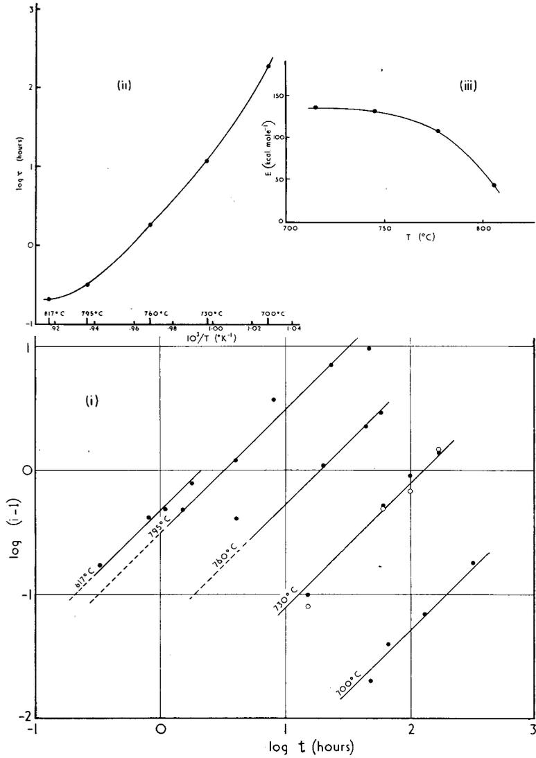
Fig. 2. (i) Plot of  $i-1 = kt$ ;  $\bullet$  refers to  $1.1 \cdot 417 \cdot \frac{1}{2}$ ,  $\circ$  refers to  $0.1 \cdot 417 \cdot \frac{1}{2}$ . (ii) Plot of  $\log \tau = E/RT + B$ . (iii) Plot of activation energy against temperature.
