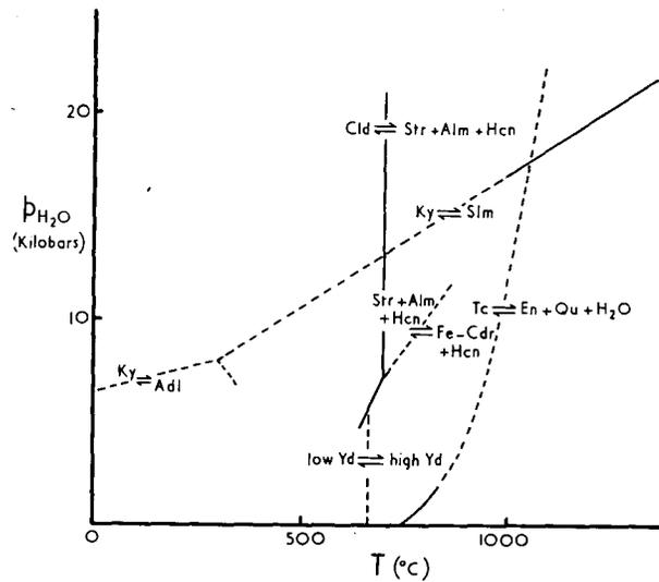
FIG. 5.  $p_{\text{H}_2\text{O}}$ - $T$  diagram illustrating the stability relations of yoderite. Key: Adl, andalusite; Alm, almandine; Cld, chloritoid; En, enstatite; Fe-Cdr, iron-cordierite; Hcn, hercynite; Ky, kyanite; Qu, quartz; Slm, sillimanite; Str, staurolite; Tc, talc; Yd, yoderite.
