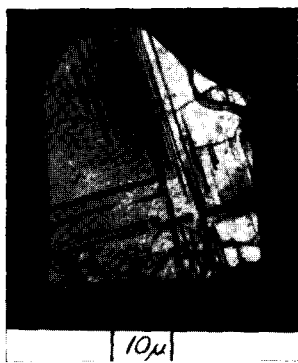
FIG. 1. Photomicrograph (crossed polars) of clinobisvanite cleavage flake showing lamellar twinning and cross hatching structure.
