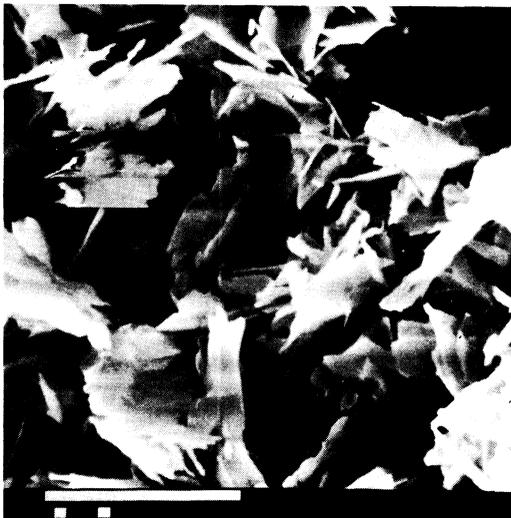
FIG. 1. Secondary electron photomicrographs of dypingite. Bar = 10  $\mu\text{m}$ .
