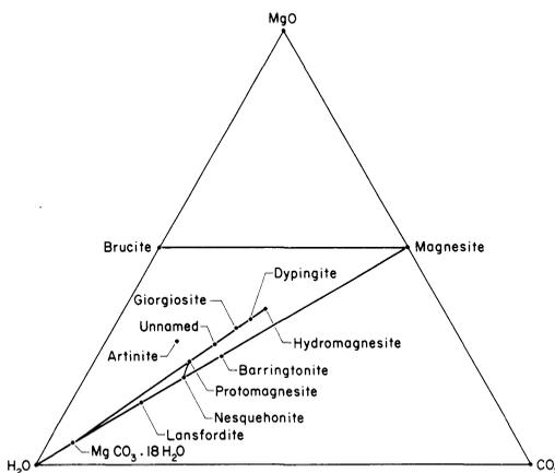
FIG. 4. The hydrated magnesium carbonate minerals in the MgO-CO<sub>2</sub>-H<sub>2</sub>O system.
