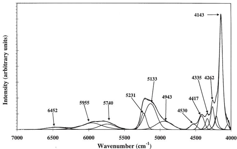
FIG. 7. NIR spectrum of conichalcite in the 4000 to 7000  $\text{cm}^{-1}$  region.
