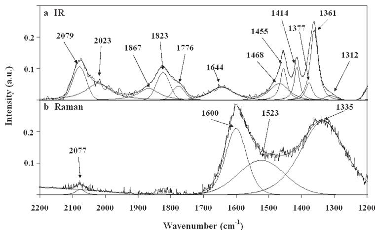
FIG. 3. Raman and IR spectra of conichalcite in the 2200–1200  $\text{cm}^{-1}$  region.
