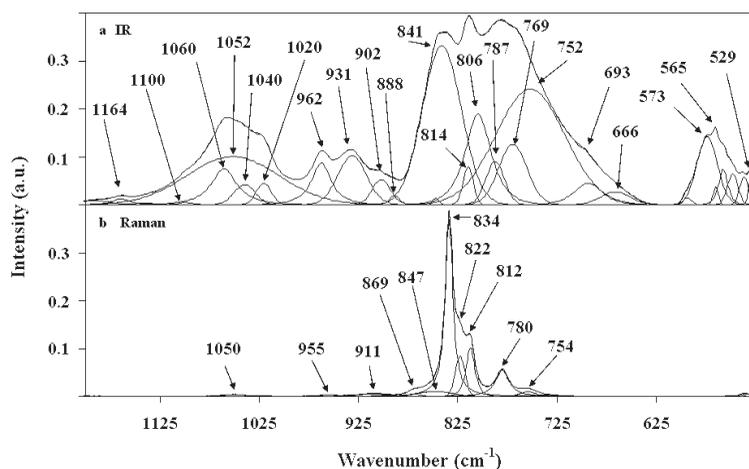
FIG. 4. Raman and IR spectra of conichalcite in the  $(\text{AsO}_4)^{3-}$  and  $(\text{PO}_4)^{3-}$ -stretching region.
