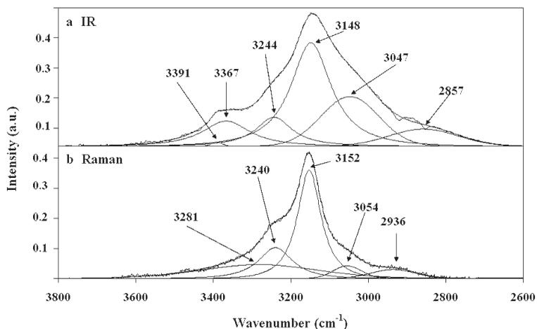
FIG. 2. Raman and IR spectra of conichalcite in the OH-stretching region.
