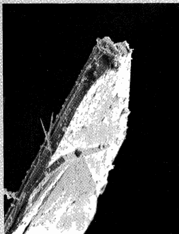
Figure 5. (top left) Ludlockite: crystal on (011), showing multiple twinning. SEM, 2000x
