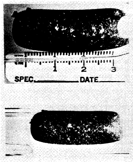
Fig. 2. \text{Cu}_{2.00115}\text{S} composition showing the effect of heating to 608^\circ for 1.3 hours. The upper picture (with cm scale) shows sample after equilibration at 100^\circ (no whiskers). The lower picture shows the presence of numerous fine copper whiskers, particularly along the bottom edge of the sample.
