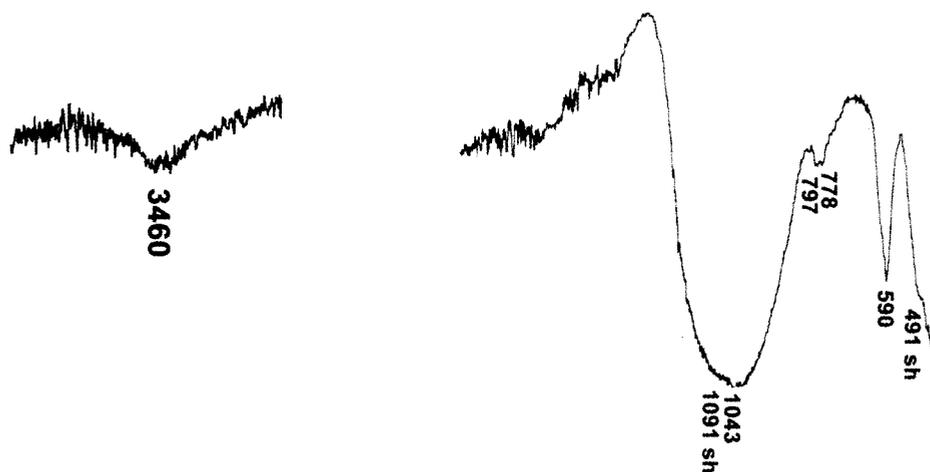
FIG. 1. The IR-spectrum of arapovite (Specord-75IR, the KBr tablet with mineral). Analyst Atali A. Agakhanov
