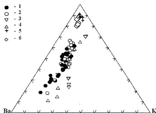
FIG. 1. The ratios of barium, strontium, and potassium (in *apfu*) in lamprophyllite from lujavrite-malignites complex rocks of Khibiny massif: lujavrites (1); «malignites-L» (2); «malignites-U» (3); «porphyric malignites» (4); and nepheline syenites of Khibiny massif (5); lujavrites of differentiated complex and eudialyte lujavrites of Lovozero massif (6)
