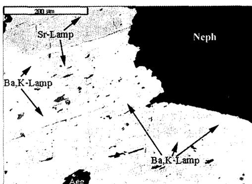
FIG. 3. The replacement of primary strontium lamprophyllite by barium-potassium lamprophyllite during K,Si-metasomatism in «malignites-U» (image in reflected electrons, scanning electron microscope JSM-5300, IGEM RAS). Ba-lamp — high-barium lamprophyllite; Sr-lamp — strontium lamprophyllite; Neph — nepheline; Aeg — aegirine
