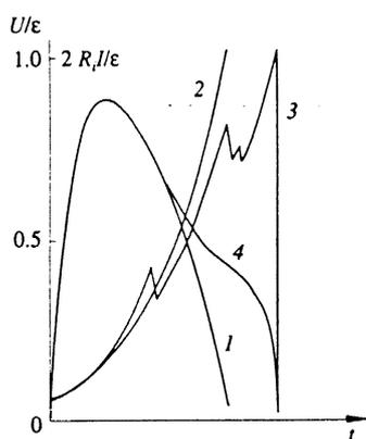
FIG. 3. Time dependence of arc current (1, 4) and voltage on the arc (2, 3): 1, 2) theory; 3, 4) experiment.
