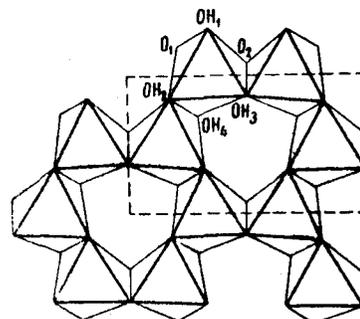
Fig. 4. Octahedral grid in kaolinite.
