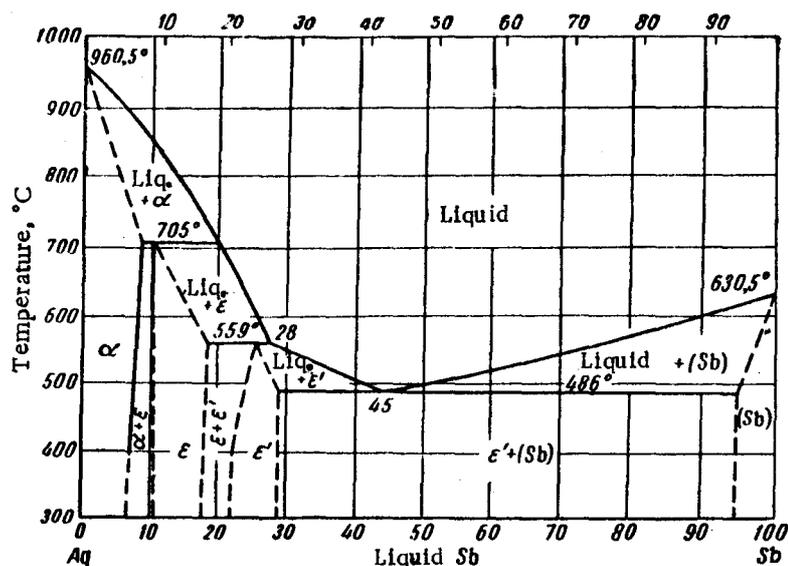
Fig. 1. Phase diagram of the Ag-Sb system
