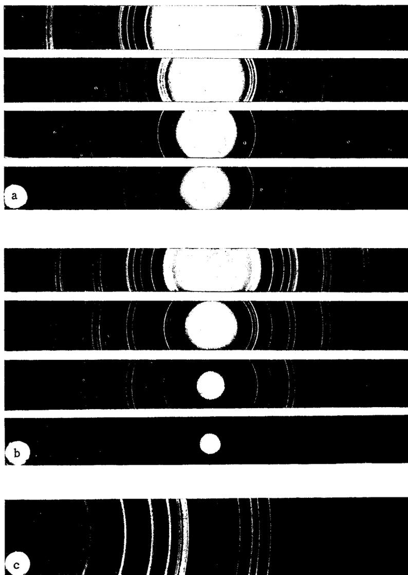
Fig. 4. Comparison of portions of two electron diffraction patterns of  $\epsilon$ - and  $\epsilon'$ -phases: a)  $\epsilon$ -phase, b)  $\epsilon'$ -phase, c) electron diffraction pattern of the  $\epsilon'$ -phase magnified 2.6 times.
