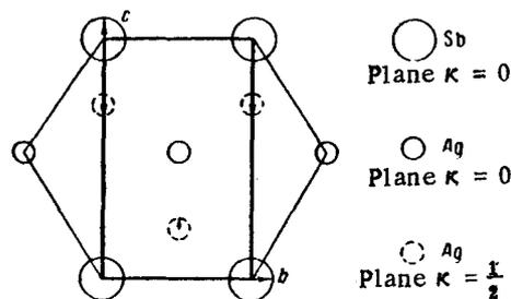
Fig. 3. Projection of the structure of the  $\epsilon'$ -phase on the (yz) plane. The arrows indicate the directions of displacement of the Ag atoms in the ordering process.
