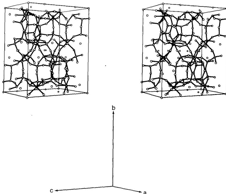
Fig.1. Stereoscopic view of the emeleusite structure. Lines are drawn from oxygen to silicon and iron, while there are no lines from oxygen to lithium (small spheres) and sodium
