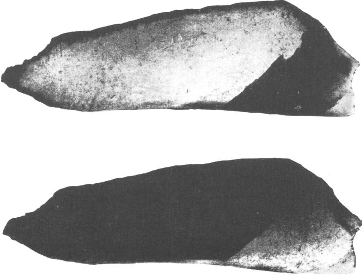
FIG. 5. Photographs taken at different angles of the smaller polished and etched surface ( $3 \times 1$  cm.) of the Hoba meteoric iron, showing the oriented sheen. Photographs by H. G. Herring.  $\times 3$ .
