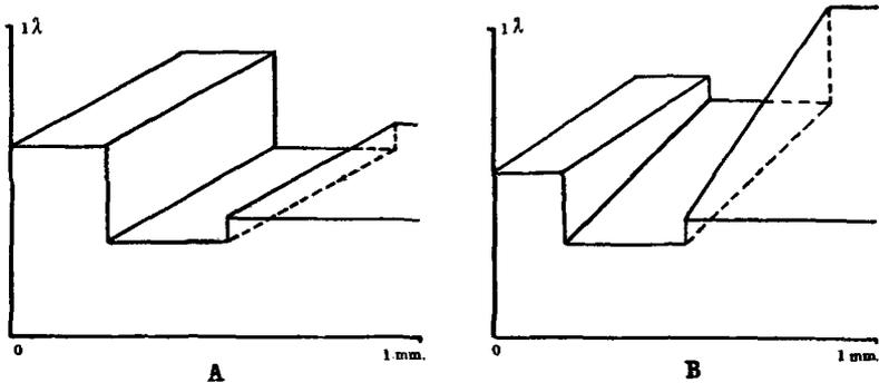
TEXT-FIG. 1. Diagram of cleavage surfaces. A, natural mica; B, synthetic mica.
