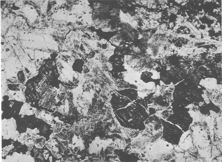
FIG. 1. Neptunite in quartz-bearing syenite, Carlingford. Ordinary light, \times 20 .
